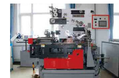
焊机 Three-piece can welder
